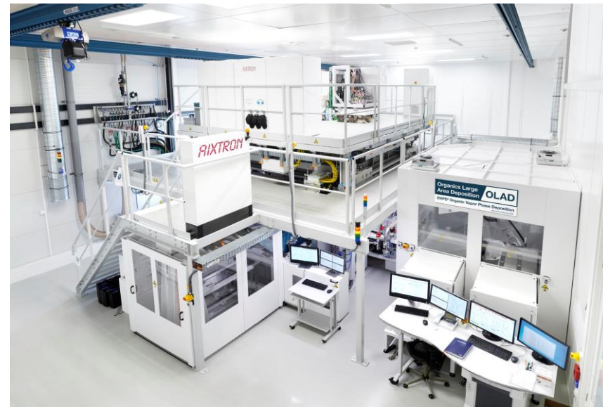
OVPD demonstrator OLAD (Organic Large Area Demonstrator) (optimized for Generation 8.5 substrate sizes)
